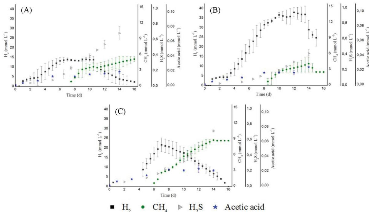
**Figure 3** Temporal profiles of  $H_2$ ,  $CH_4$ ,  $H_2S$  and Acetic acid concentrations for conditions: C1, 2.0 g cellulose  $L^{-1}$  (A); C2, 5.0 g cellulose  $L^{-1}$  (B) and C3, 10.0 g cellulose  $L^{-1}$  (C)
