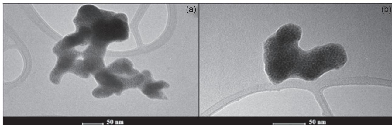
Figure 1. Transmission Electron Microscopy of NPs-Co
