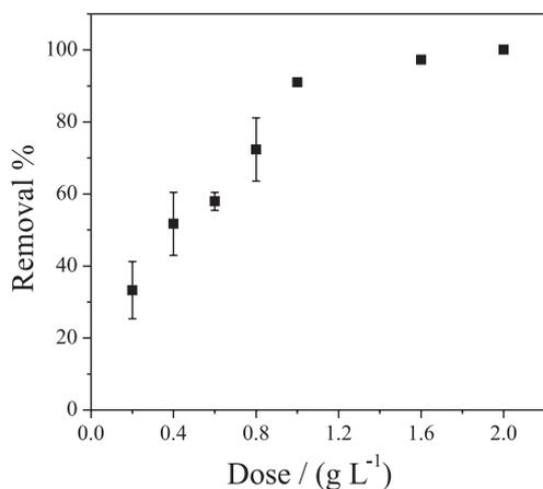
Figure 8. Effect of the dose of NPs-Co on the removal of Cr(VI). Experimental conditions:  $C_{Cr(VI)} = 40.0$   $\text{mg L}^{-1}$ ; volume of solution =  $20.0$   $\text{mL}$ ; system temperature =  $25$   $^{\circ}\text{C}$ ; without pH adjustment ( $8.5$ ); dose of NPs-Co =  $1.0$   $\text{g L}^{-1}$ ; reaction time =  $10$  hours
