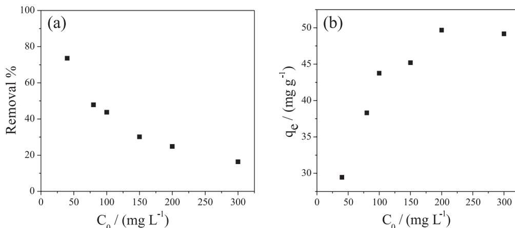
Figure 7. (A) Effect of the initial concentration Cr(VI) on the removal process; (B) Effect of the initial concentration Cr(VI) on the removal capacity. Experimental conditions:  $C_{Cr(VI)} = 40.0, 80.0, 100.0, 150.0, 200.0$  and  $300.0$   $\text{mg L}^{-1}$ ; volume of solution =  $20.0$   $\text{mL}$ ; system temperature =  $25$   $^{\circ}\text{C}$ ; dose of NPs-Co =  $1.0$   $\text{g L}^{-1}$ ; without pH adjustment ( $8.5$ ); reaction time =  $10$  hours
