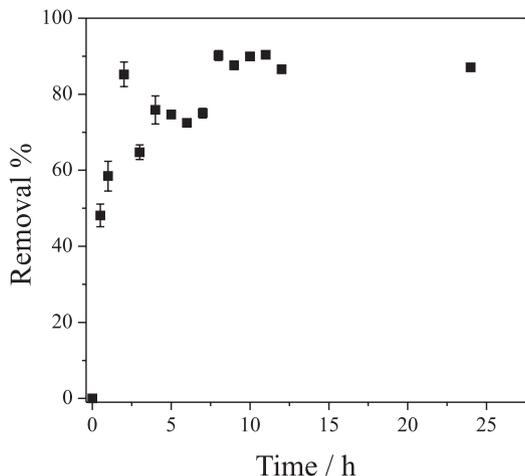
**Figure 4.** Reactional equilibrium time between NPs-Co and Cr(VI). Experimental conditions:  $C_{Cr(VI)} = 40.0 \text{ mg L}^{-1}$ ; volume of solution = 20.0 mL; system temperature = 25 °C; dose of NPs-Co = 1.0 g L<sup>-1</sup>; without pH adjustment (8.5); reaction time = 24 hours
