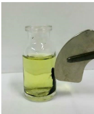
Figure 1S. NPs-Co in the presence of an external magnetic field
