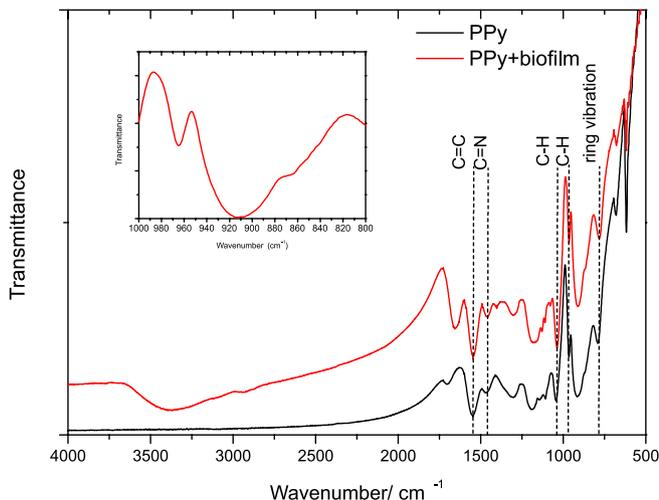
**Figure 3.** FTIR spectrum of polypyrrole and polypyrrole+ biofilm of *S. aureus* (in the inset is shown the region around  $860 \text{ cm}^{-1}$  for sample PPy+biofilm)
